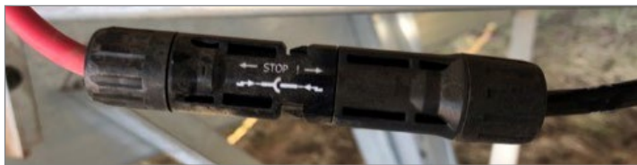
A mismatched MC4 and MC4-compatible connector in the field at a site with extensive connector failures.
