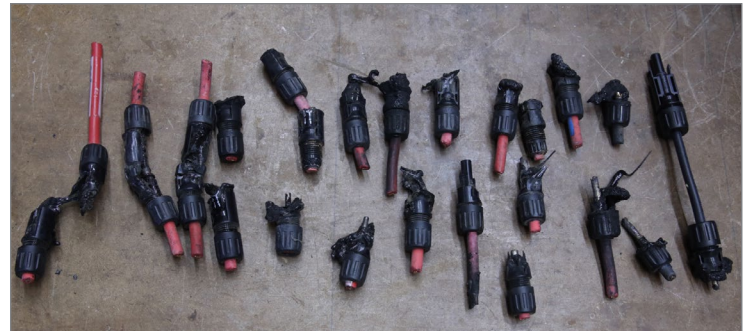
The sample of failed connectors above melted due to high temperature operation in the field. PVEL removed the devices from the field for testing and root cause failure analysis.
