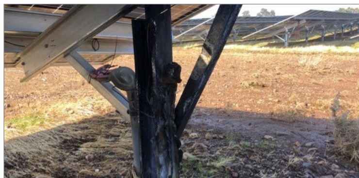
A single overheated connector caused this catastrophic failure. Per PVEL's testing, installation error is likely the root cause.
