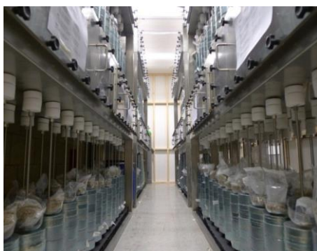
Figure 10. Full-scale test rig for 30 mbar(g). Inside the test rigs, the materials are exposed to various gases.
