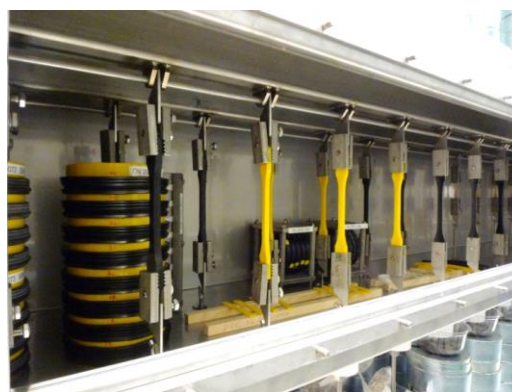
Figure 9. Constant load experiments on PE dumbbell samples and constant strain experiments on NBR samples that have been placed over oversized pipes.
