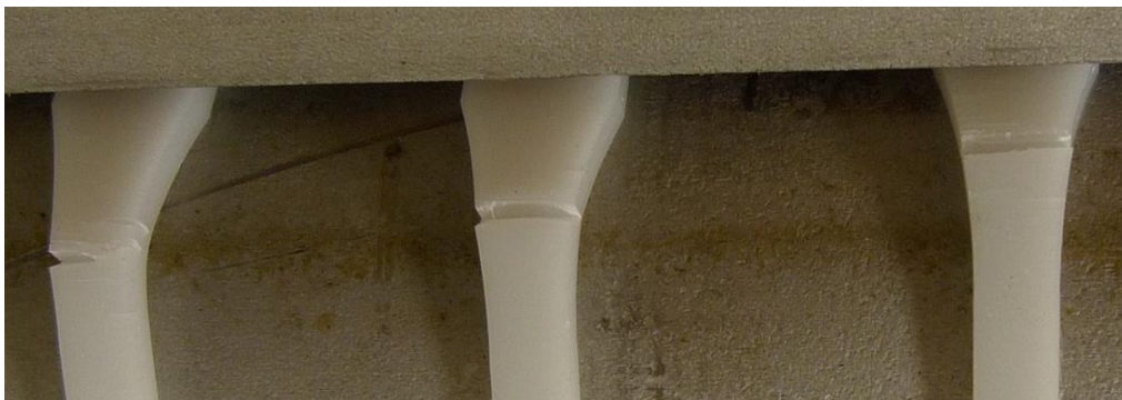
Figure 34. Three cPOM dumbbells, still mounted in the test rig, which broke during the exposure period of 600 days to humid 3 ppm HCl vapour.
