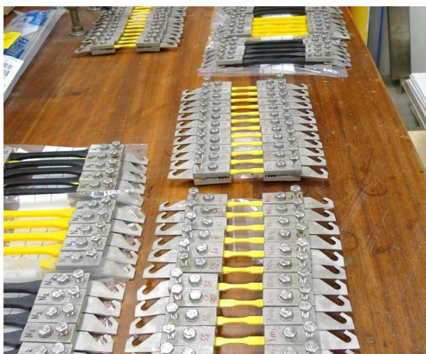
Figure 6. PE and PVC dumbbell samples clamped for ESC experiments.
