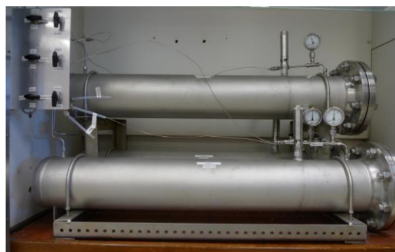
Figure 11. Full-scale test rig for 8 bar(g). Inside the test rigs, the materials are exposed to various gases.
