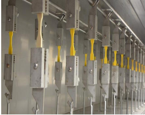
Figure 7. Constant load experiments on PVC dumbbell samples.
