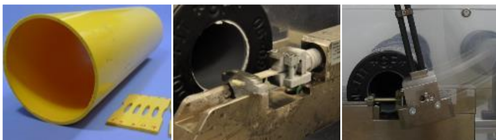
Figure 40. PVC-HI pipe with dumbbell-shaped specimens.
