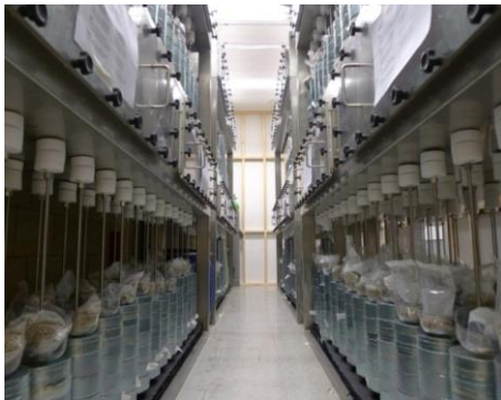
Figure 9. Full-scale test rig for 30 mbar(g). Inside the test rigs, the materials are exposed to various gases.
