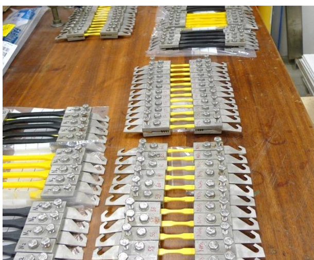
Figure 5. PE and PVC dumbbell samples clamped for ESC experiments.
