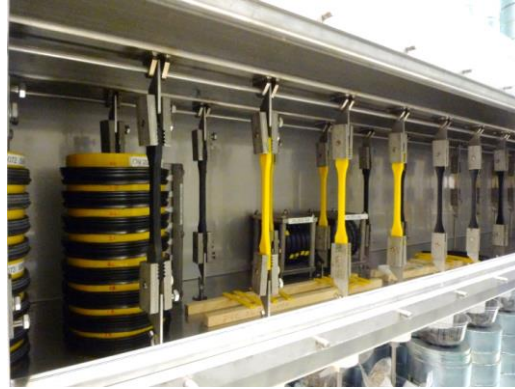
Figure 8. Constant load experiments on PE dumbbell samples and constant strain experiments on NBR samples that have been placed over oversized pipes.
