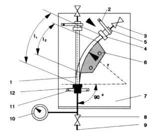
Figure 1 — Bending template
