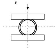
Figure 1 - test set-up for compression
