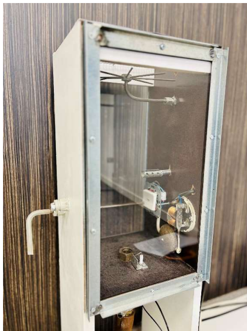
Figure 2: Test setup to visualize hydrogen flammability. Source: Kiwa Technology
