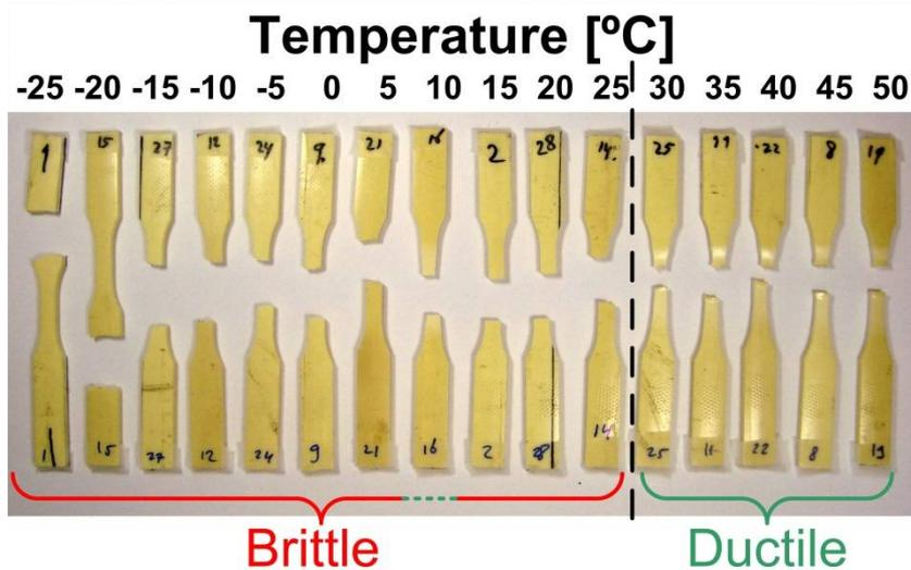
Figure 3B test bars of a poor quality pipe with a high  $T_{BD}$ .
