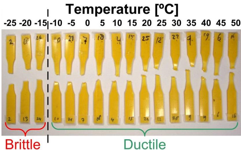
Figure 3A: test bars of a good quality pipe with a low  $T_{BD}$ .
