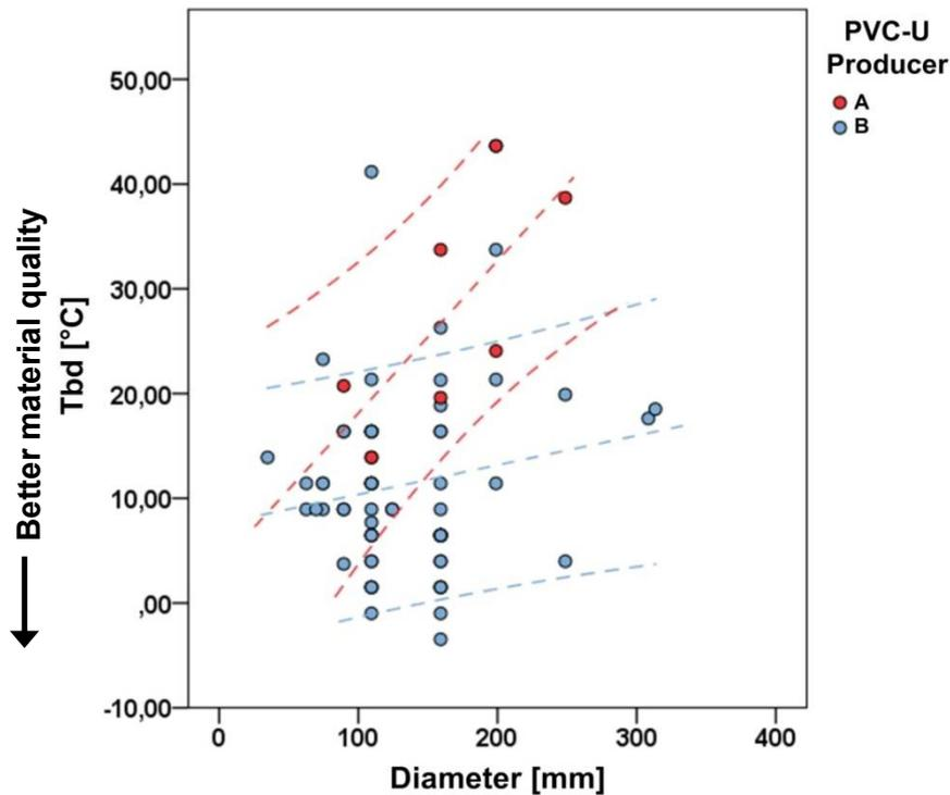
Figure 9: Brittle-ductile-transition-temperature ( $T_{BD}$ ) of old PVC-U pipes versus diameter differentiated by producer.
