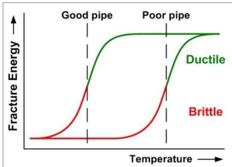
Figure 2: Schematic graph of the brittle-ductile-transition-temperature for a good and a poor quality PVC pipe.
