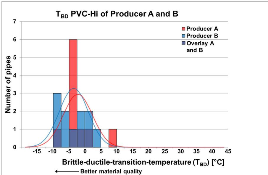
Figure 11: No significant difference in  $T_{BD}$  between old PVC-Hi of producer A and B.
