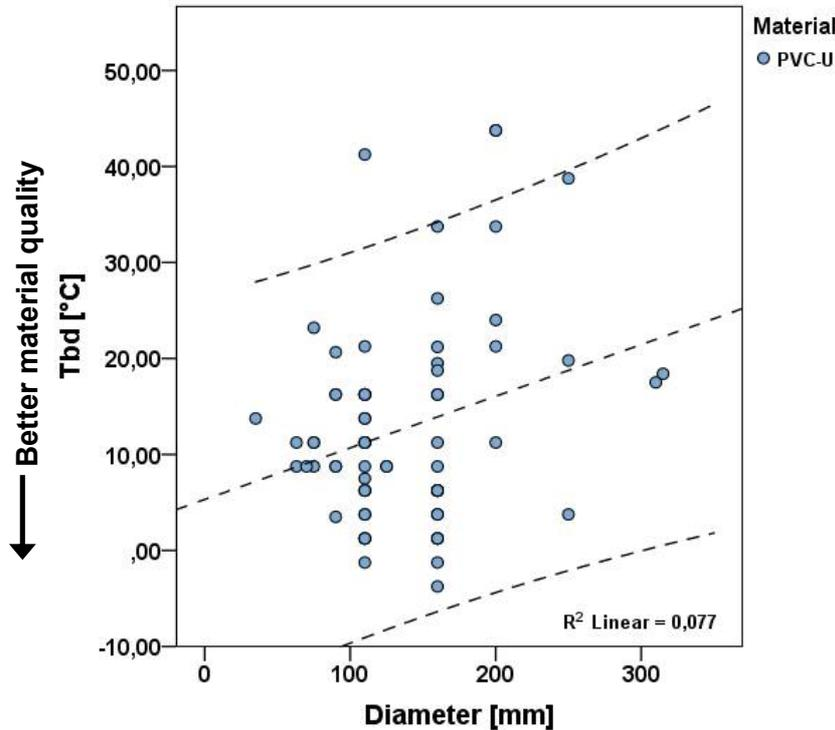
Figure 7: Trend between the brittle-ductile-transition-temperature ( $T_{BD}$ ) and the diameter of old PVC-U pipes.
