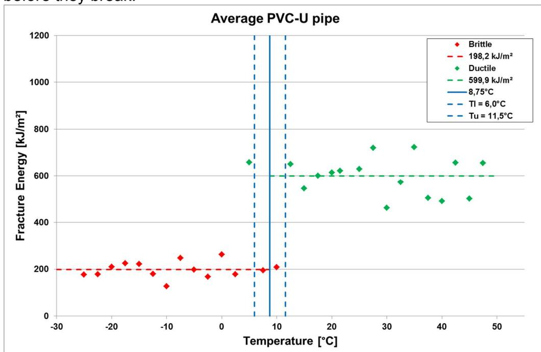
Figure 4: An average PVC-U pipe with a  $T_{BD}$  of  $8,75^{\circ}\text{C}$ .
