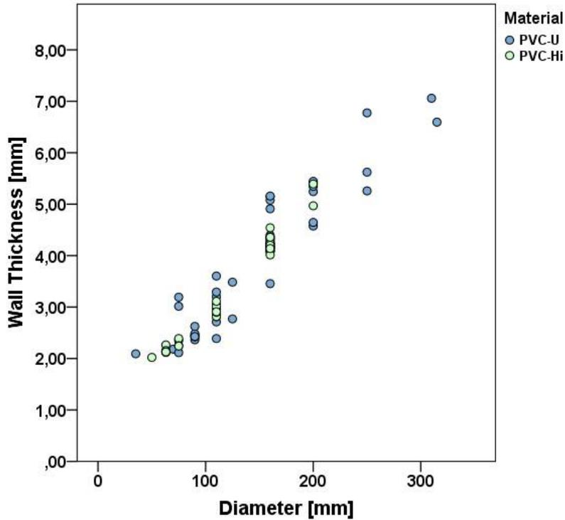
Figure 8: Wall thickness versus diameter of the analyzed PVC pipes.
