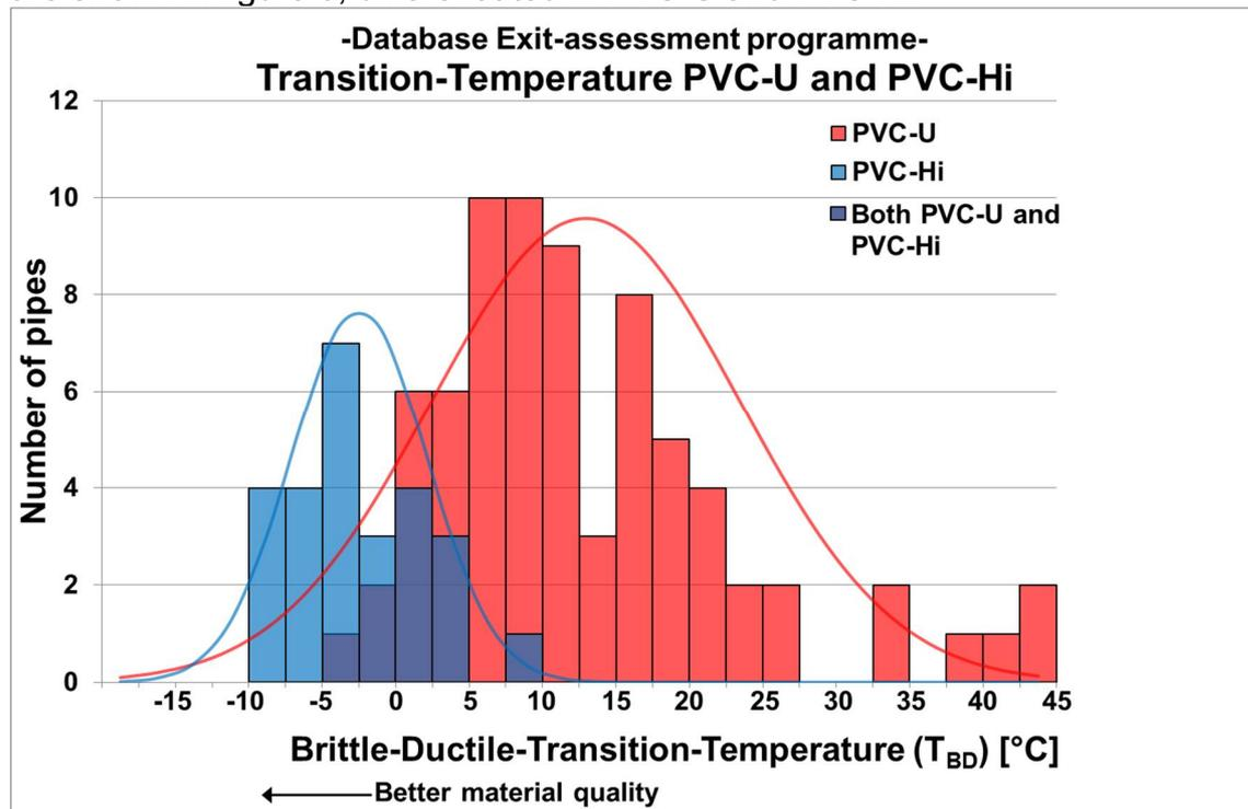
Figure 6: Histogram  $T_{BD}$  (brittle-ductile-transition-temperature) of PVC-U and PVC-Hi.
