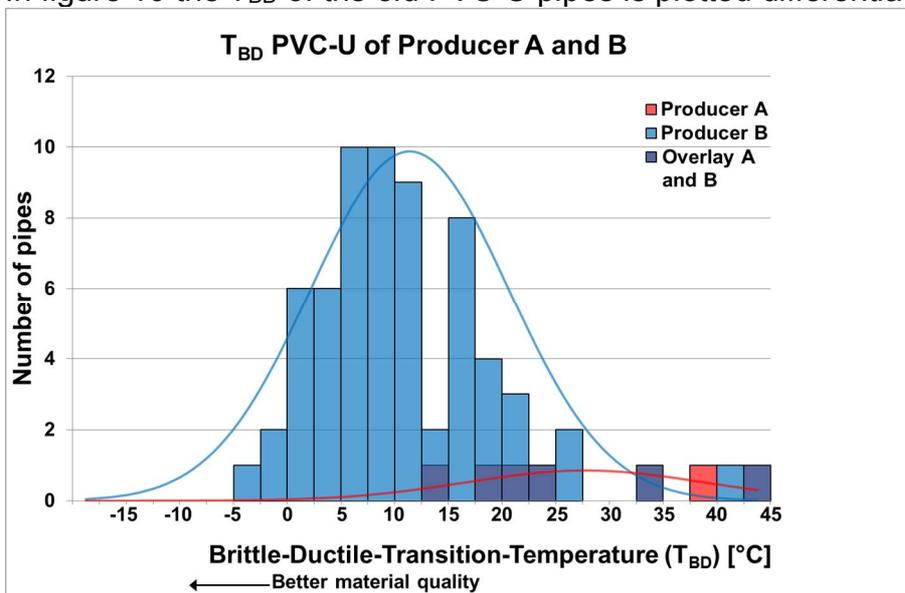
Figure 10: Significant difference in  $T_{BD}$  between old PVC-U pipes of producer A and B.
