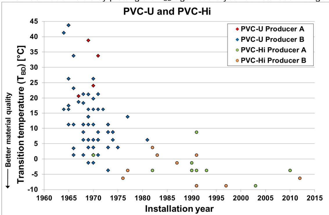
Figure 12: Brittle-ductile-transition-temperature versus installation year.
