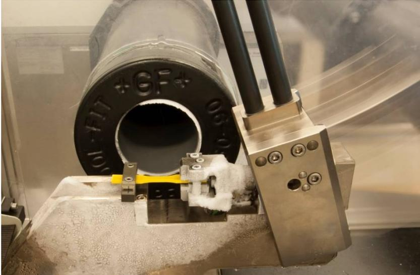
Figure 1: Experimental setup: standard impact tester with added heating and cooling.
