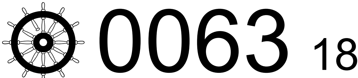
Figure 6: Marking for marine equipment approved by Kiwa and affixed in 2018.
