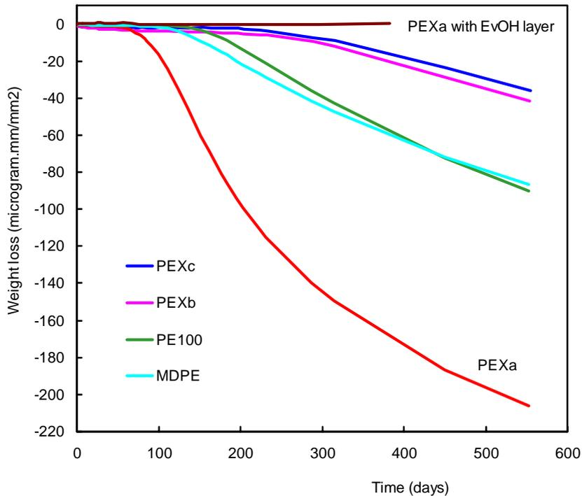
**Fig. 1** Normalised weight losses by permeation of odorant (THT) through the pipe walls of different PE and PEX pipes. Measurements carried out with saturated odorant vapour in air ( $72,400 \text{ mg/m}^3$ ).
