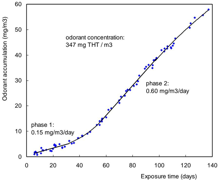
**Fig. 2** Permeation through a 18 mm diameter PEXa pipe without EvOH layer, filled with natural gas containing 347 mg/m<sup>3</sup> THT odorant and accumulation within a casing pipe.
