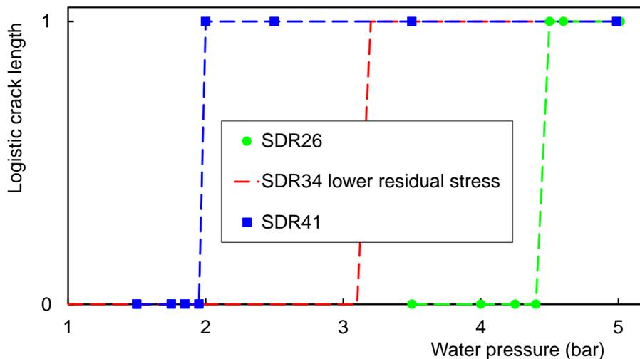
Figure 13. Prediction of the logistic crack length of SDR34 segments with the model, assuming a lower residual stress. Here,  $P_C$  increases from 1.95 to 3.1 bars. The curves of the SDR41 and SDR26 segments are not influenced.
