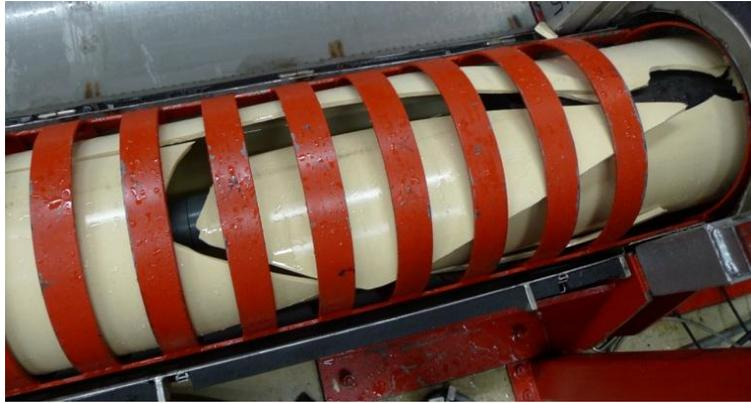
Figure 5. RCP after the S4 test above  $P_C$  on a water-filled 315 mm PVC pipe segment. The crack propagated further to the left, almost reaching the end of the segment (not shown).
