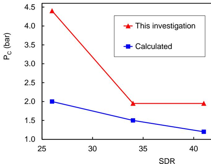
Figure 9. Influence of the SDR on the  $P_C$  of 315 mm PVC pipes in the hydrostatic S4 test and values calculated using the method proposed by Leavers et al [7-12].
