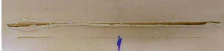
Figure 6. External pipe surface of an "inert" segment without crack initiation. The knife bounced once thus creating a second smaller notch, also in axial direction.
