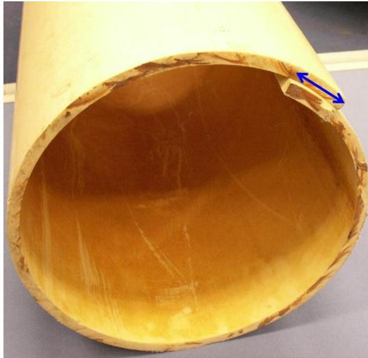
*Figure 10. Overlap of the pipe wall (blue arrow) in tangential direction after RCP. From this overlap, or after cutting a bar in axial direction out of an intact pipe, the shrinkage in the tangential direction is calculated as a percentage (Table 1).*
