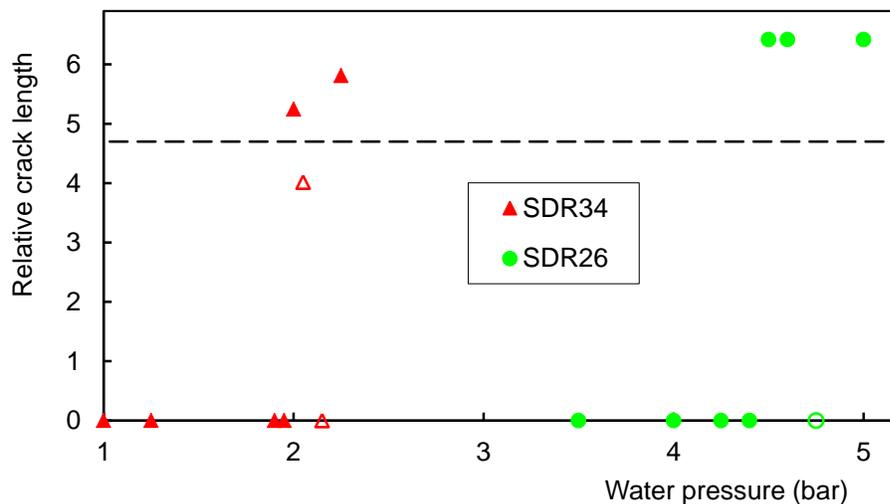
Figure 8. As Figure 7, for SDR34 and SDR26 pipes. Open symbols: to be removed from the  $P_C$  determination as prescribed by ISO<sup>[6]</sup>. SDR34:  $P_C = 1.95$  bar, SDR26:  $P_C = 4.40$  bar.
