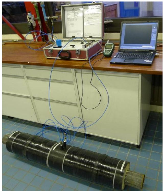
Figure 4. A district heating pipe joint is pressurised; the pressure and flow are measured.
