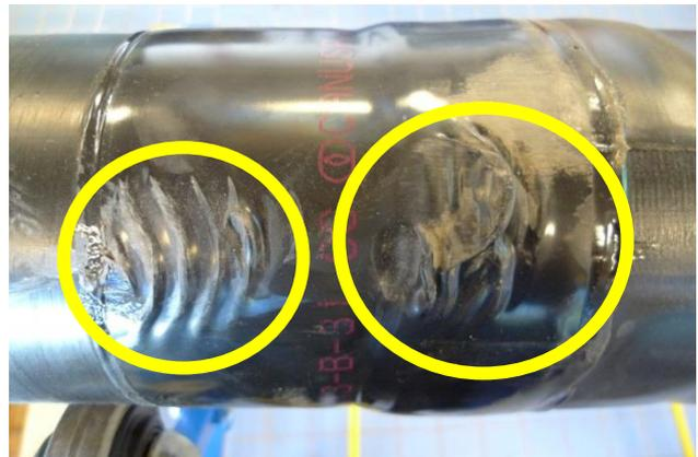
Figure 6. Wrinkles in the collar of a PEX shrink sleeve.
