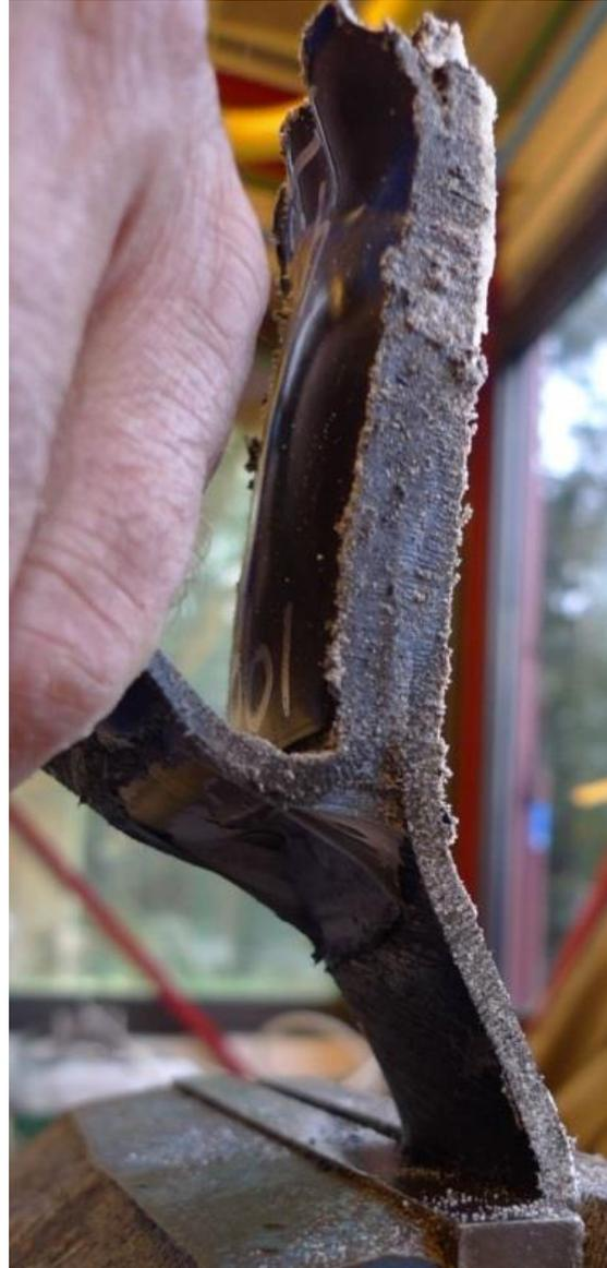
Figure 16. The bonding between the PEX shrink sleeve and the PE casing is strong enough to withstand manual peeling.
