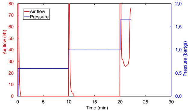
Figure 9. Air flow (lower trace, red) and pressure (upper trace with steps, blue) during a pressure test with air until failure of the PE shrink joint. Below 1 bar(g) the air flow is 0 l/h after an initial peak as the pressure increases. At 1.5 bar(g) the air flow increases considerably, indicating a leak.
