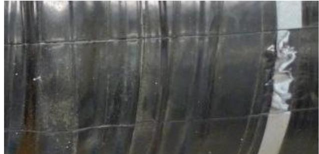
Figure 12. These tapes were strongly bonded to the PE casing. The edge on the right side shows unsuccessful attempts to detach the tape.
