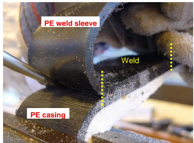
Figure 17. The weld is strong enough to withstand manual peeling.
