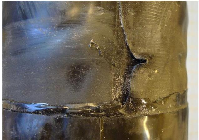
Figure 5. Fold in PEX shrink sleeve.
