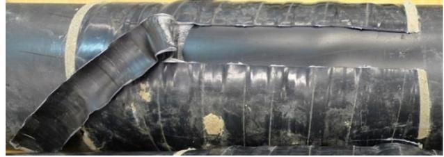
Figure 11. A poorly abraded joint, resulting in a low tape bonding strength. The tapes were easily peeled away from the PE casing and shrink sleeve manually. The quality of this water barrier is therefore low.
