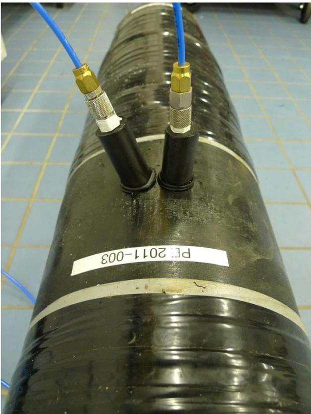
Figure 3. Connections to a district heating pipe joint using two hollow PE rods to perform the leak tightness test.
