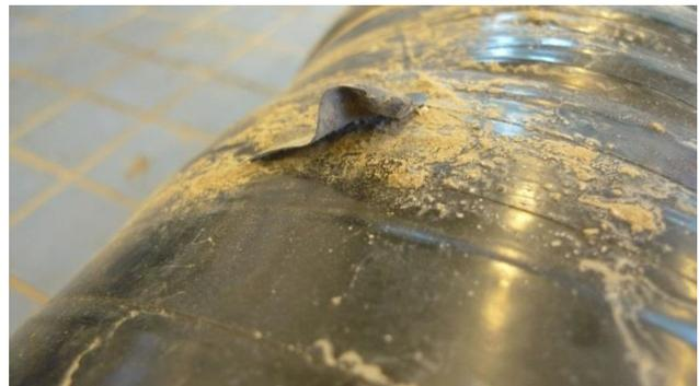
Figure 7. A tape ending halfway across the taped area. This causes a weak spot in the system.
