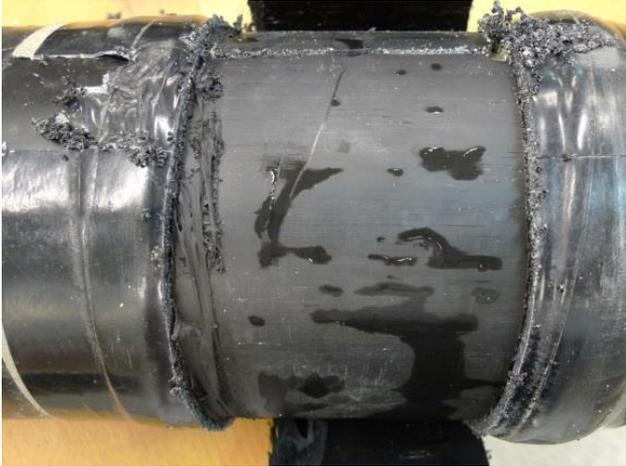
Figure 18. PE shrink sleeve removed to show water trapped in the joint.
