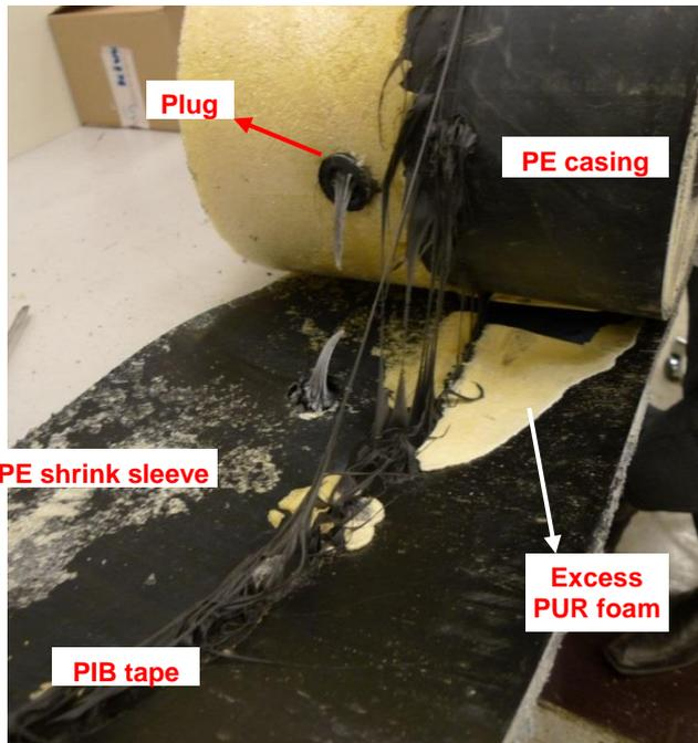
Figure 19. PUR foam has flowed beyond the PIB tape barrier, creating a failure in the first water barrier.
