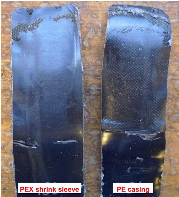
Figure 14. There is no bonding strength between the PEX shrink sleeve and PE casing, probably due to insufficient heating.
