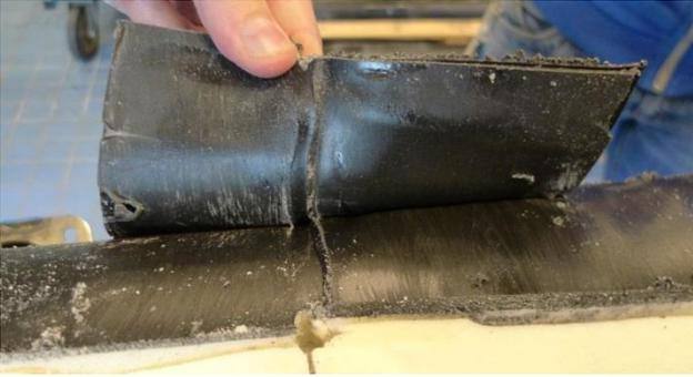
Figure 13. The collar of this PEX shrink joint could easily be detached manually from the casing and the PEX shrink sleeve.
