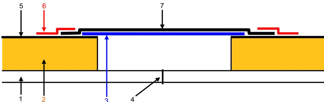
Figure 2. Cross-section of a joint (schematic). (1) Service pipe (steel), (2) Insulation (PUR), (3) Optional shrink film, (4) Weld in the steel pipe, (5) Casing (PE), (6) Shrink collar (PEX) or tapes (butyl rubber, Densolen N8 and black Denso foil) and (7) Shrink sleeve (PEX or PE) or welded sleeve (PE).
