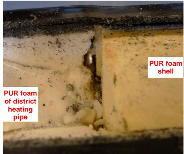
Figure 20. PUR foam is cut very irregularly, so that the PUR foam shell does not fit tightly, which leads to large gaps.
