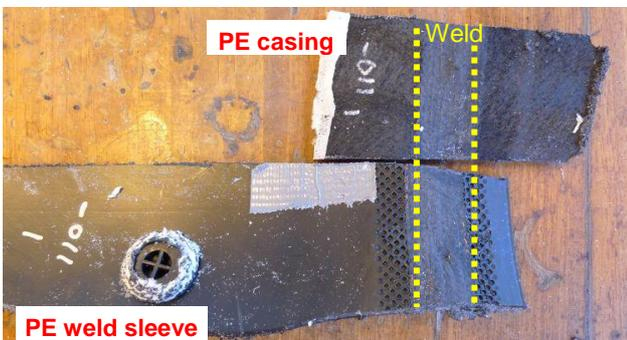
Figure 15. The PE weld sleeve and the PE casing are not properly fused. The PE weld sleeve could therefore easily be manually peeled away from the PE casing.
