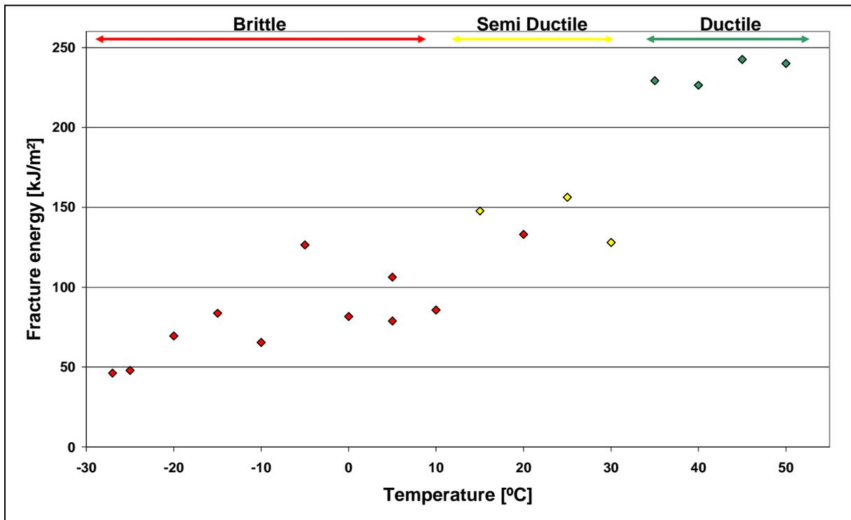
Figure 8: Combination of tensile impact test results and fracture behaviour for pipe A.
