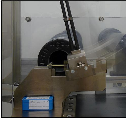
**Figure 2: The tensile-impact tester about to hit a test bar.**
