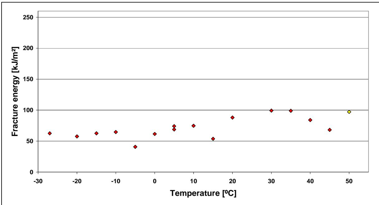
**Figure 11: Combination of tensile-impact test results and fracture behaviour for pipe B.**
