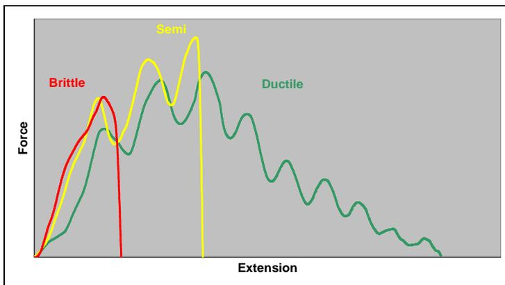
**Figure 6: Three types of fracture; brittle, semi-ductile and ductile.**
