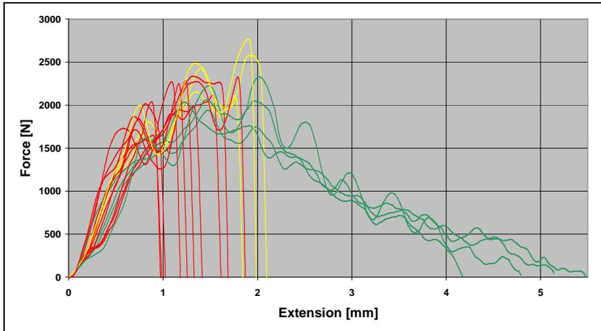
**Figure 5: Force-extension curves for the individual test bars of pipe A.**
