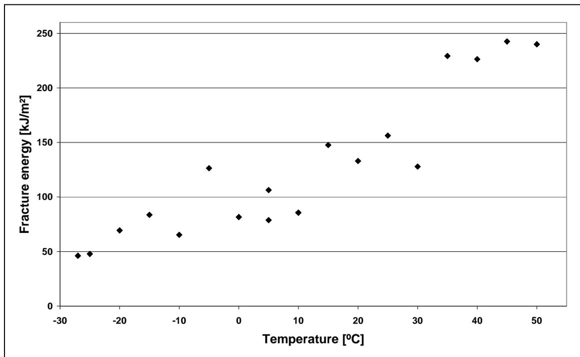
**Figure 4: Tensile impact graph of pipe A (PVC-U) at various temperatures.**
