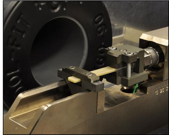
**Figure 3: Air from the tube on the left keeps the test bar at the desired temperature.**
