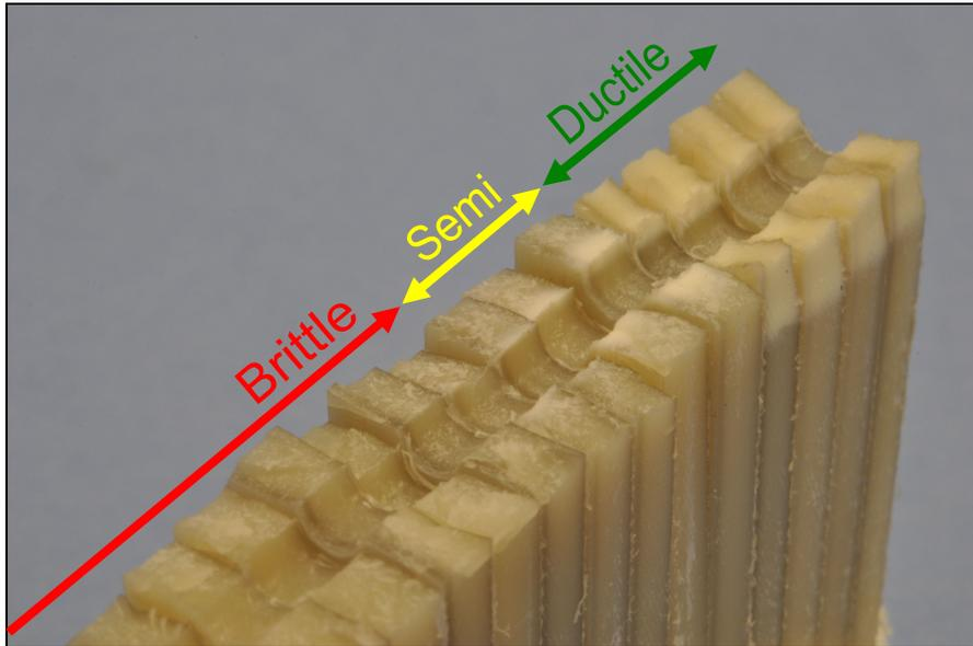
Figure 7: By visual characterization three types of fracture are found.
