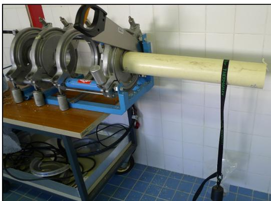
**Figure 13: The saw-test performed on a PVC-U pipe**
