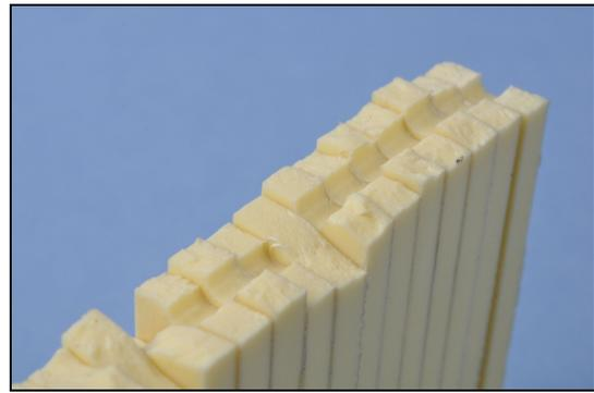
**Figure 10: The fractured samples of pipe B.**
