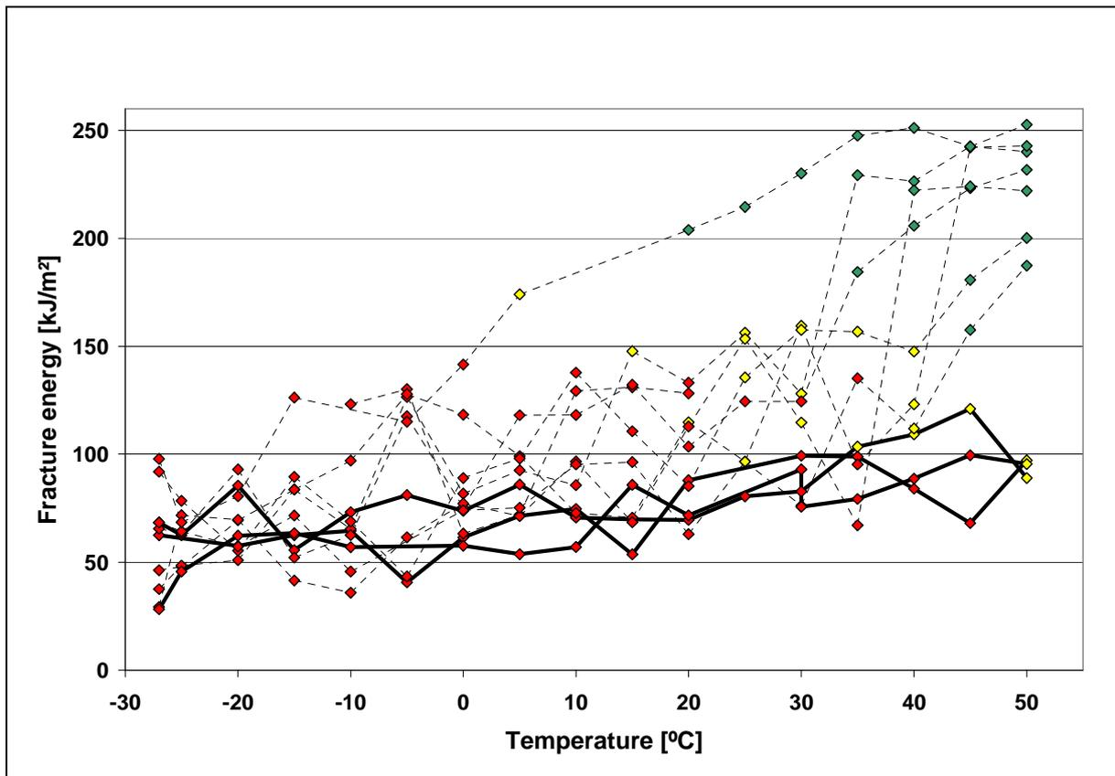
**Figure 12: Tensile impact test results of 11 different pipes from at various temperatures**
