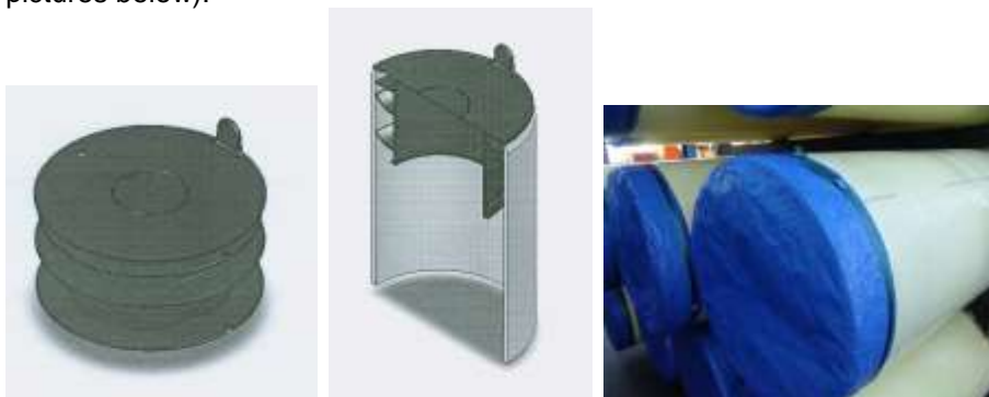
Left: end cap with flaps. Right: fiber reinforced cover in combination with adhesive tape.
